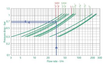
Reference values: Upstream pressure = 8 bar Downstream pressure = 3 bar
