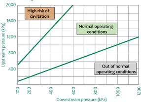
In order to minimise the risk of cavitation in the reducing valve, which could cause malfunctions with the risk of erosion in the seal area, vibration and noise, you are strongly advised to refer to the operating conditions specified in the diagram.
